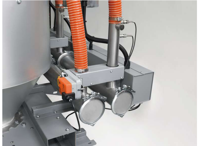
(a) Process air flow management system
